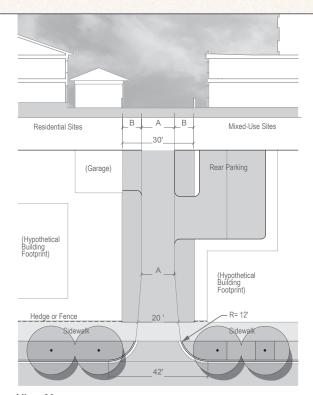
Alley: 30 ROW: 30 feet. (A) Paved Area: 14-22 feet, (B) Pervious Side Areas 4-8 feet (turf or pervious paving). Throat Width 20 feet, Curb Radius 12 feet. Curb extends to the Sidewalk. Utility Easements shall be provided for the entire Alley area. Comparative Pedestrian Crossing Distance 18 feet, Time 6 seconds. (All dimensions to face of curb.)
